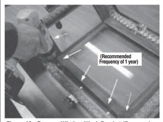
Figure 40 - Remove Window Wash Bracket (5 screws)
